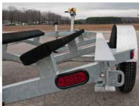
fender pads, galvanized rims, UFP torsion axles with industry-leading UFP vault hubs and much, much more. Available in single, tandem and tri-axle configurations, these Aluminum Custom Bunk Trailers offer the best the boating world has to offer.
